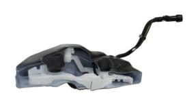
Cross-section view of the fuel tank
