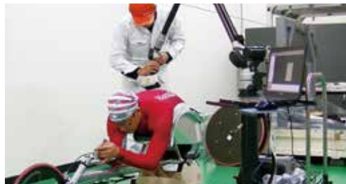
Analysis of cornering forces on frame structure
